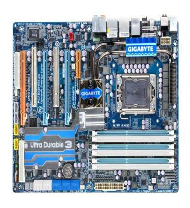
The system board connects all system components and allows input and output devices to communicate with the system unit. It is the main Switchboard of the system. They are also called main board or motherboards. The system board is the communications medium for the entire computer system.
